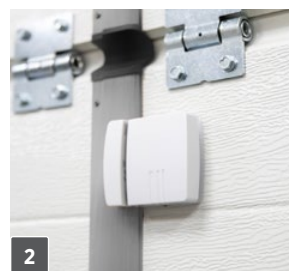
2 The wicket door opening sensor prevents activation of the garage door when the wicket door is open. The wicket door option in automatic doors includes a wicket door opening sensor.
